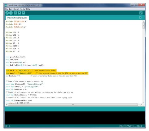
Then upload the sample code and press reset, and you can see related information shown in serial monitor.
